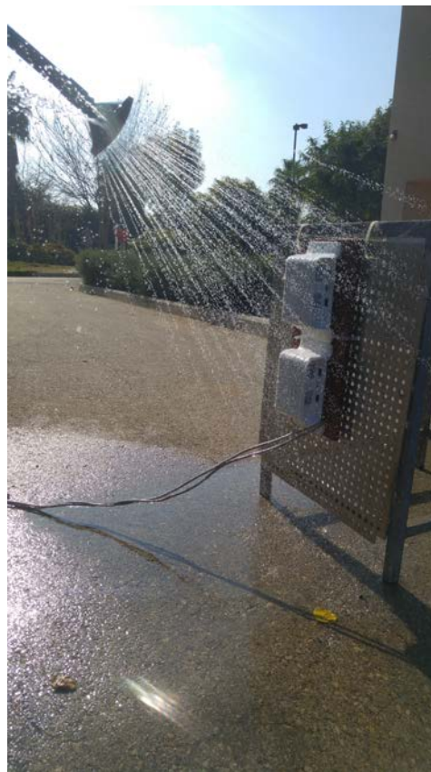
Photograph 6.4.1 The EUTs under splashing water
