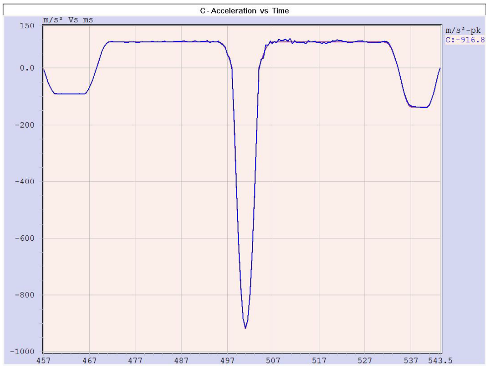
Plot 6.6.2 The negative shock pulse along vertical axis (operational)
