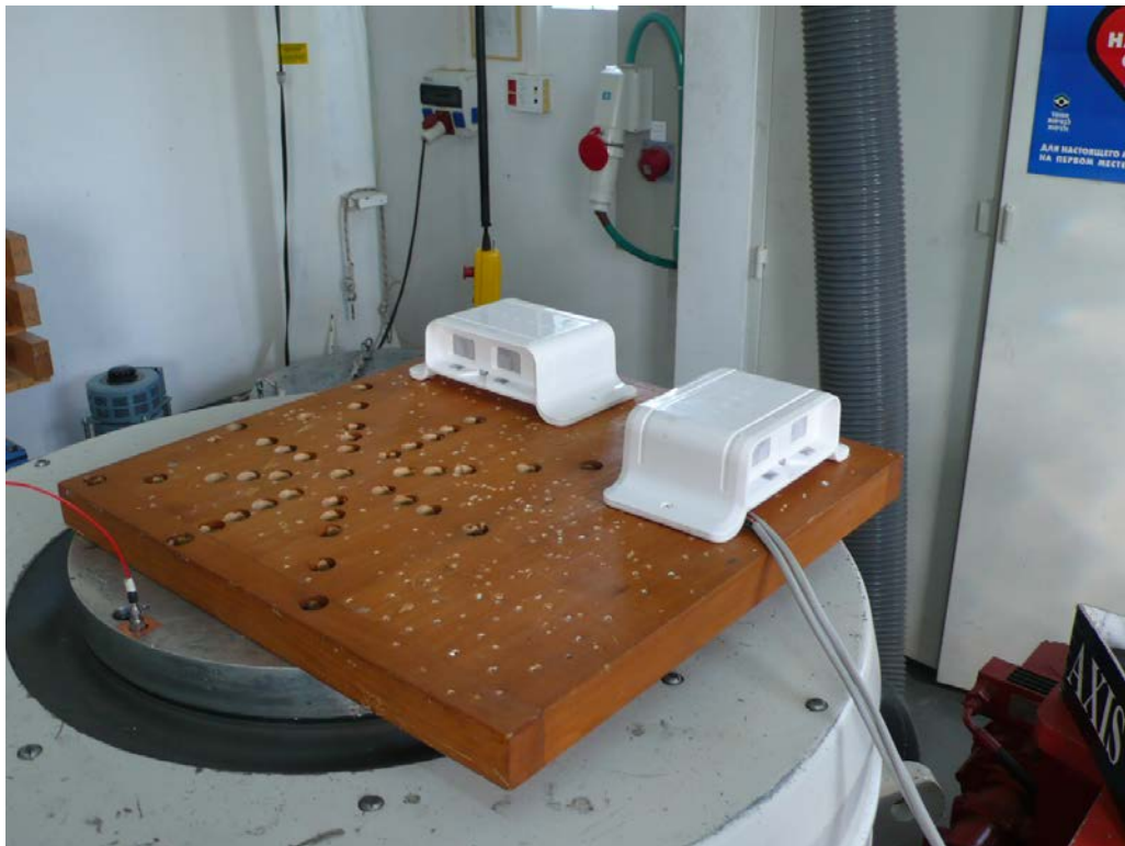
Photograph 6.6.1 Shock test setup (vertical axis)
