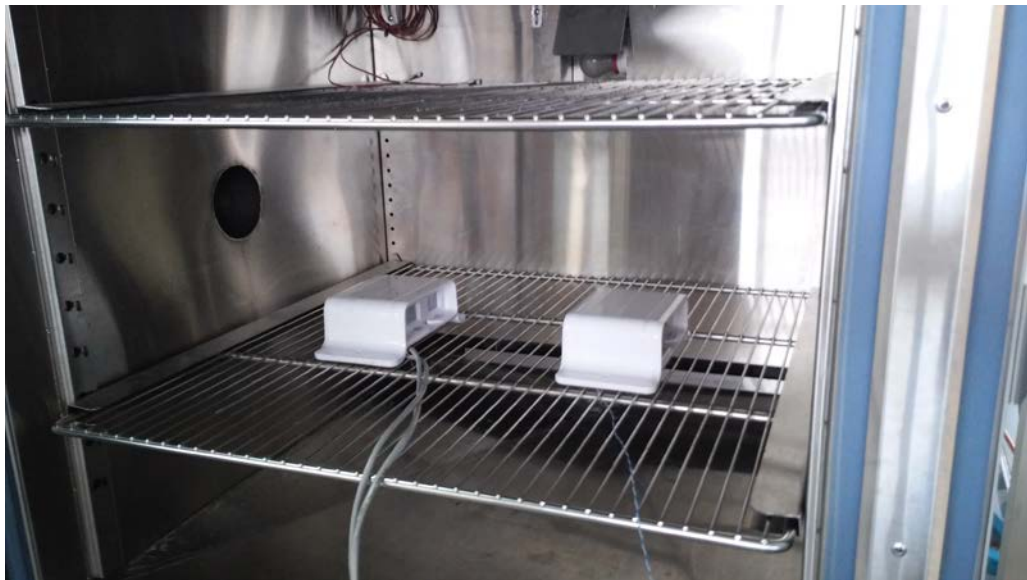
Photograph 6.3.1 The EUTs in the humidity chamber
