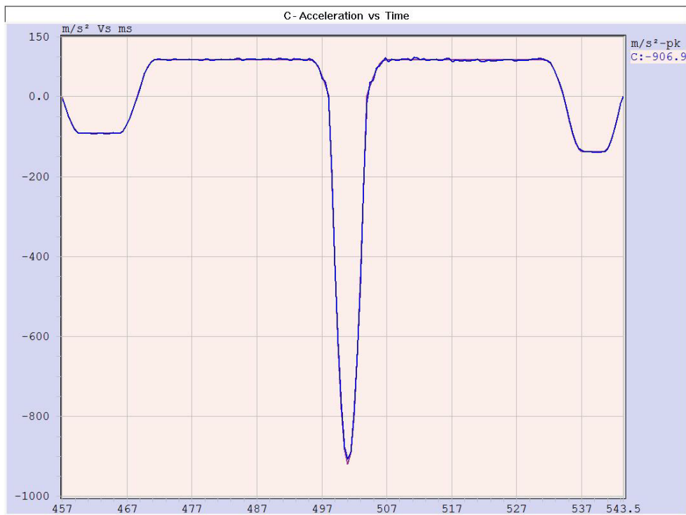
Plot 6.6.6 The negative shock pulse along longitudinal axis (Operational)
