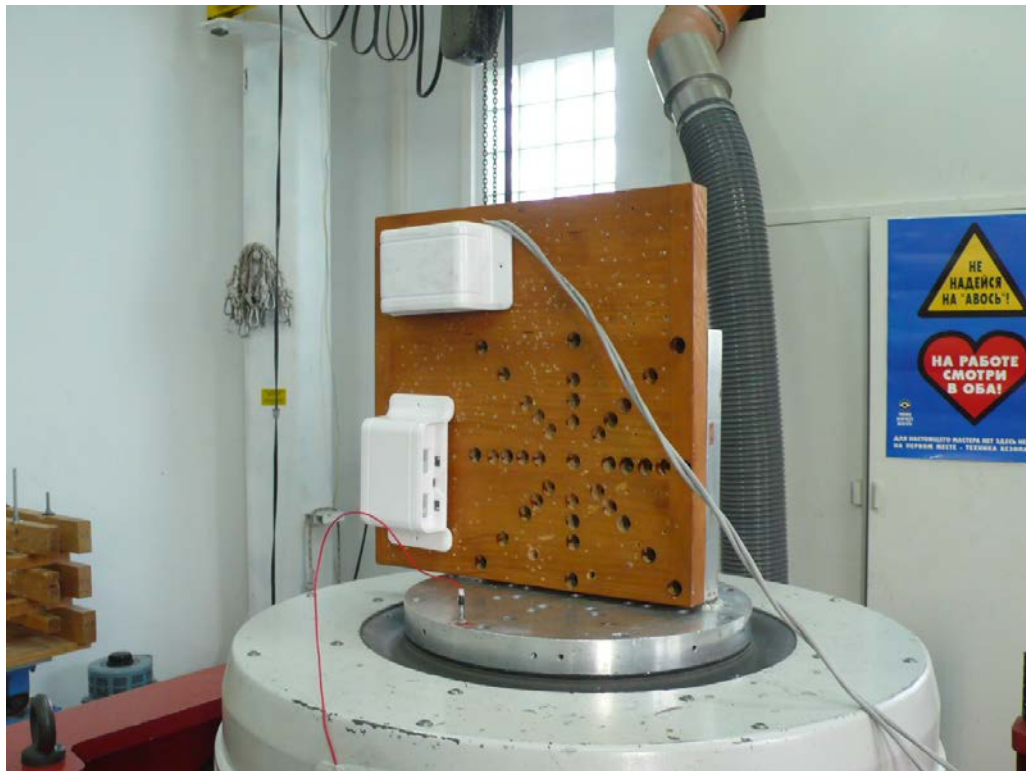
Photograph 6.6.3 Shock test setup (longitudinal axis)
