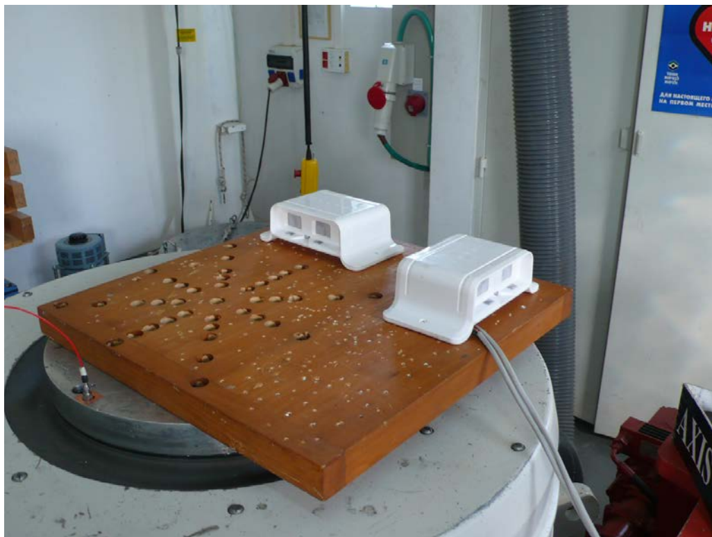
Photograph 6.5.1 Sinusoidal vibration test setup (vertical axis)
