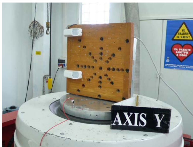
Photograph 6.10.3 Shock test setup (longitudinal axis)
