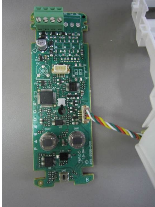
Photographs 5.1.11, 5.1.12 Wired PIR detector NV35MX internal view
