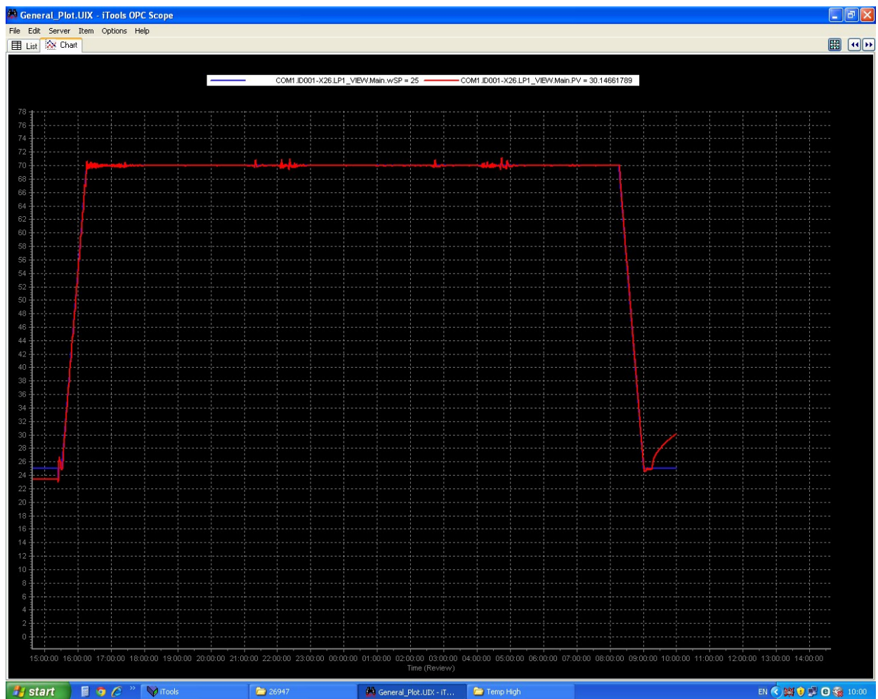
Plot 6.2.1 Temperature monitoring during the dry heat (operational) test
