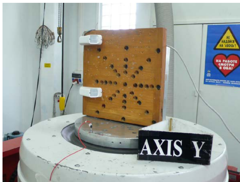
Photograph 6.8.3 Sinusoidal vibration test setup (longitudinal axis)
