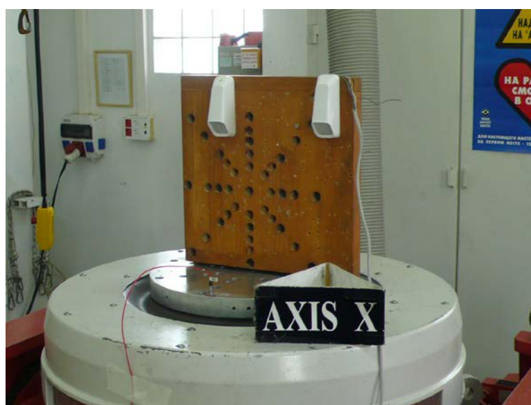
Photograph 6.9.2 Sinusoidal vibration test setup (transverse axis)
