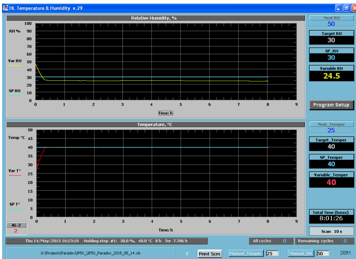
Plot 6.7.1 Temperature - humidity monitoring during dust test
