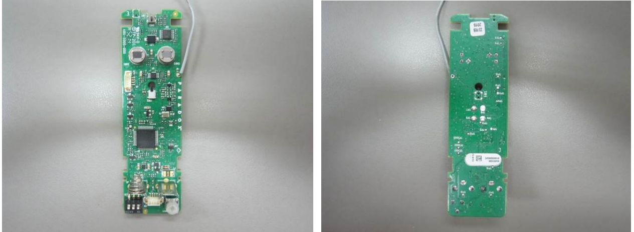
Wireless PIR detector NVR35M internal view
