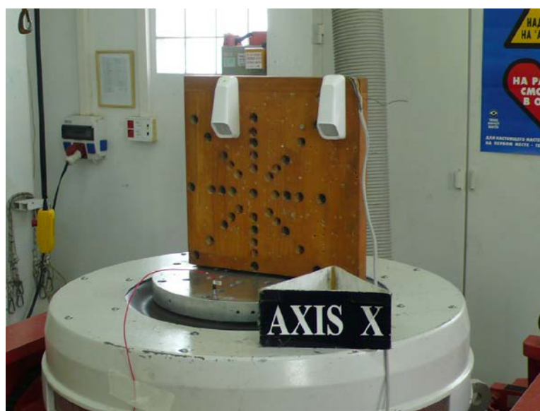
Photograph 6.8.2 Sinusoidal vibration test setup (transverse axis)
