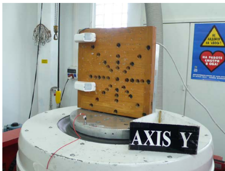
Photograph 6.9.3 Sinusoidal vibration test setup (longitudinal axis)
